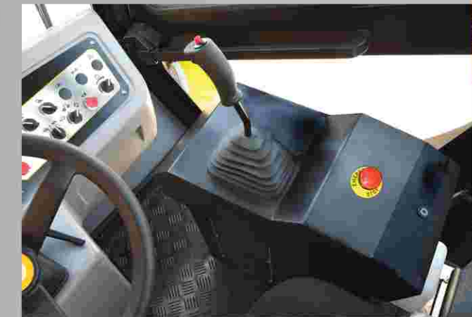
Drive control lever and potentiometers which regulate engine rpm.
