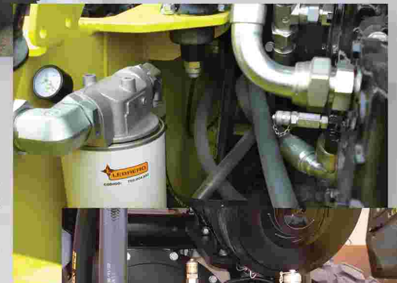
Location of hydraulic filters, hydraulic pumps with pressure inlets, more accessibility and easier.
