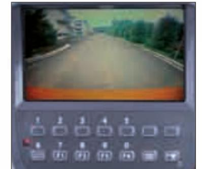
The widescreen color LCD, teamed up with the rear view camera on the counterweight, gives the operator unobstructed rearward viewing. The rear view camera automatically works when traveling, and can also be manually turned on with a select switch on the monitor.
